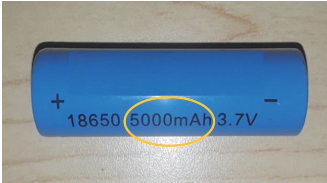
Figure 5. Manufacturer's label displaying cell capacity of 5000 mAh on the cell. Upon lab testing, measured cell capacity was only 1200 mAh.
