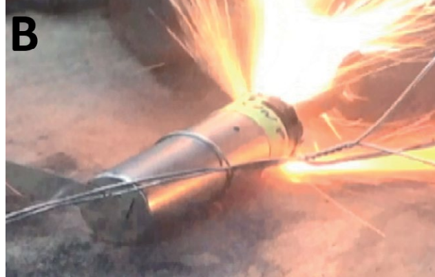
Figure 4. Comparison of overcharge test on authentic (A) and low-quality (B) cell showing difference in safety of these cells. Electrolyte leak, high heat and fire is observed in case of low-quality cell.
