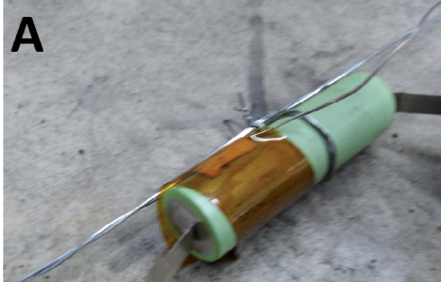
Figure 4. Comparison of overcharge test on authentic (A) and low-quality (B) cell showing difference in safety of these cells. Electrolyte leak, high heat and fire is observed in case of low-quality cell.
