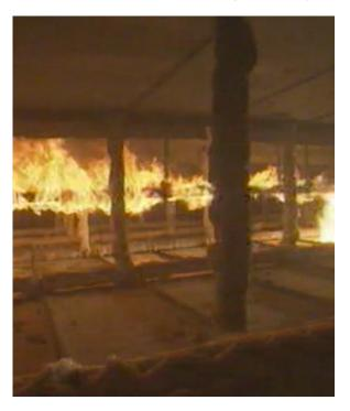
**UL Solutions Certification, Factory and Market Surveillance**On Feb. 7, 1978, UL Solutions issued a fact-finding report of our investigation comparing flame propagation and smoke development tests on communications cables in various test geometries. The report was used to develop a test method for determining adequate fire resistance and low smoke-producing characteristics of cables to be adopted by the NEC.
