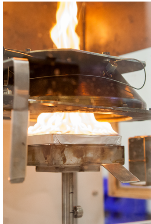
Cone calorimeter testing
