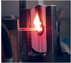
IEC Glow-Wire Flammability/ IEC Glow-Wire Ignition
