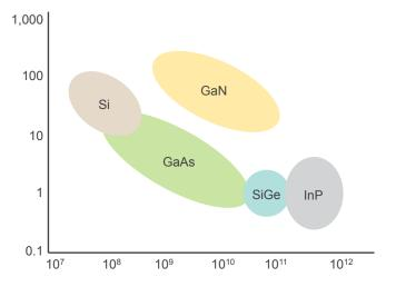
Figure 3: Working frequencies and power of various high-frequency semiconductor technologies<sup>4</sup>
