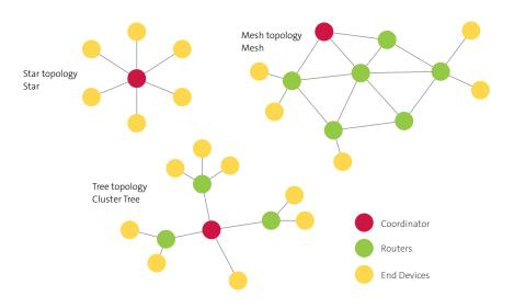
Figure 4: Network topology for mobile communications<sup>5</sup>
