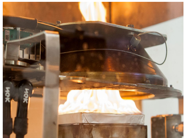
Cone calorimeter testing
