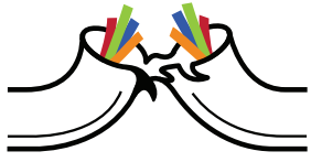
Breakage of conductors
