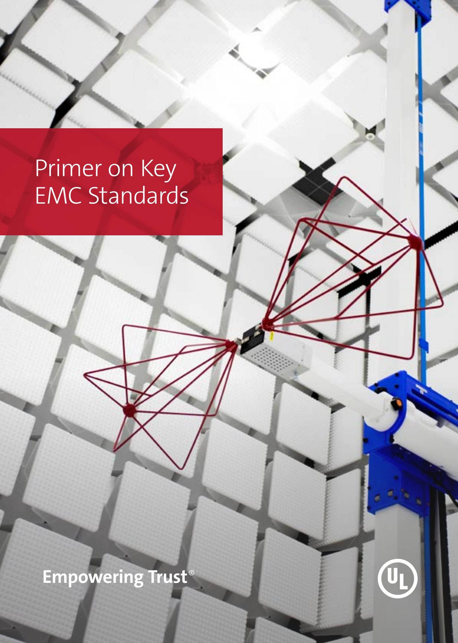
The image shows the interior of an anechoic chamber, characterized by a dense array of white, pyramidal-shaped electromagnetic absorbers designed to eliminate reflections. A red wireframe antenna structure is suspended in the center, connected to a small electronic device. To the right, a blue mechanical arm or probe is visible, extending into the chamber. The lighting is bright, creating a high-contrast environment.
