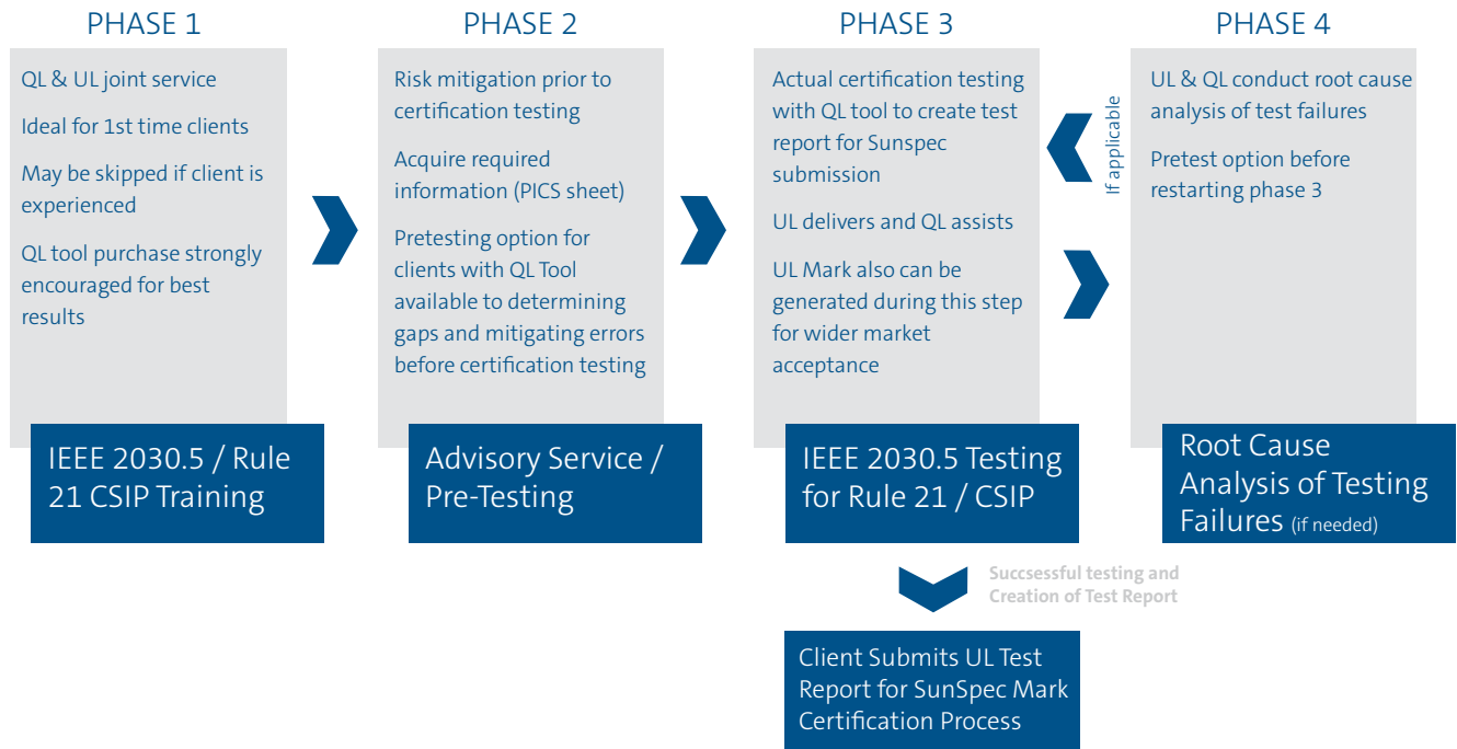
Figure 1. The combined modular UL certification process leveraging UL's collaboration with Quality Logic
